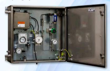
The integrity of the sampling system is as important as the analyzer itself. To sample natural gas from a pipeline, the sampling system must reduce pressure and guide the sample from the sampling point to the analyzer, leaving the mercury concentration unchanged. Plus it should show a minimum lag time and be suited to hard use in hazardous zones.
